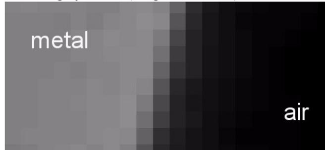
**VGStudio MAX 2.0** uses these voxels of intermediate gray value to find the surface of an object with sub-voxel precision.
