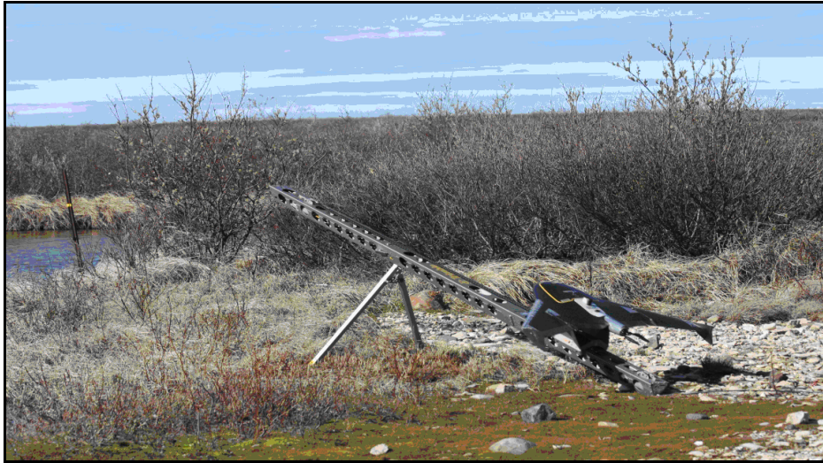
Figure 19. The Trimble-Ux5 mounted on its catapult launcher ready to launch from Nestor 2.
