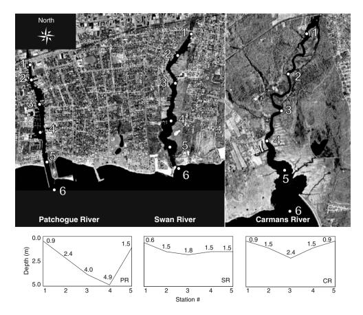
Fig. 2 Tidal sections of PR, SR, and CR; aerial digital orthophotos (New York State, 1996). *Below* Mean low tide river channel depth in meters at each tidal section station. Stations 6 have open bay characteristics
