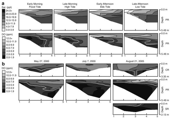
Fig. 4 Salinity and dissolved oxygen (DO) visualizations. Depth is on the *y*-axis, and station number is on the *x*-axis. The *white isoline* indicates the 5 ppm DO level. The *black regions* indicate water with a DO level of 2 ppm or lower. **a** PR tidal cycle salinity and DO collected
