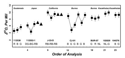
**TABLE 4.** Drift corrected oxygen isotope values ( $\delta$ 180, ‰) for jadeitite samples
