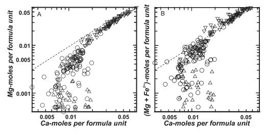
formula unit (b). The sum  $(Mg + Fe^{2+})$  shows a small excess over Ca in the range of Ca = 0.02 to 0.05. Either some of the Fe calculated by the 6 oxygen, 4 cation normalization to be  $Fe^{2+}$  is in fact  $Fe^{3+}$ , or an extremely small augite component is also present.
